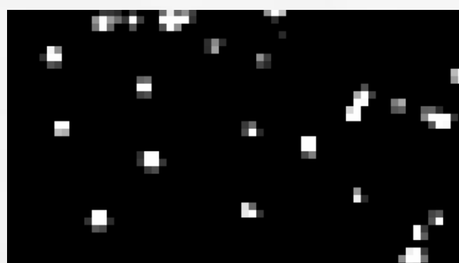
Figure 2 Beta particle signals being recorded in a CCD at room temperature
