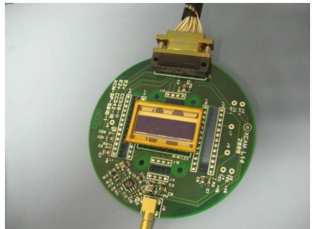
Fig 4: (Left) The CCD38 used for evaluation of high signal handling capacity CCDs, and (right) the CCD30-11 used for radiation damage studies
