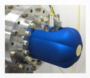
The RIXSCam™ Mini system is mounted on a 6" CF flange with the detector at a fixed gamma-angle chosen by the customer. The system has been designed to enable users to replace the detector as needed, offering a long-term, economically viable solution.
