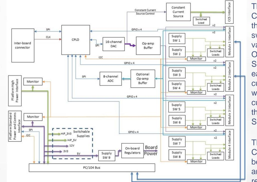
The Experiment Controllers provide the hardware to switch power rails to various parts of the **Optical and Vacuum** Subsystems and each has a constant current source circuit
