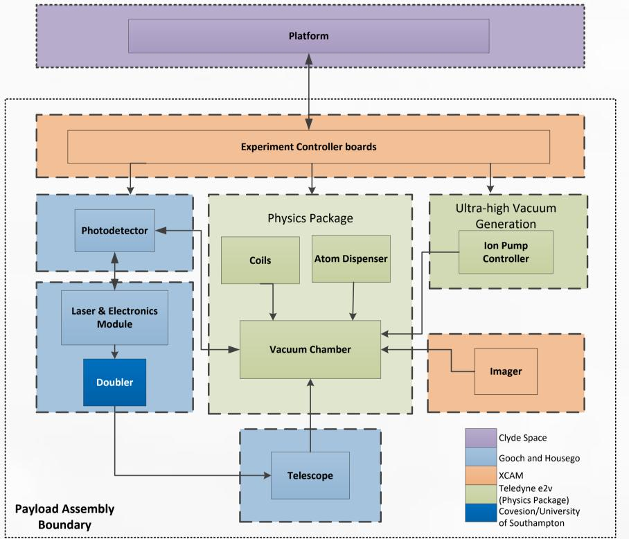
The Payload Assembly can be split into 3 subsystems; Electronics Subsystem (XCAM), Optical Subsystem (Gooch & Housego with Covesion and University of Southampton PPLN incorporated) and the Vacuum Subsystem or Physics Package (Teledyne e2v).
