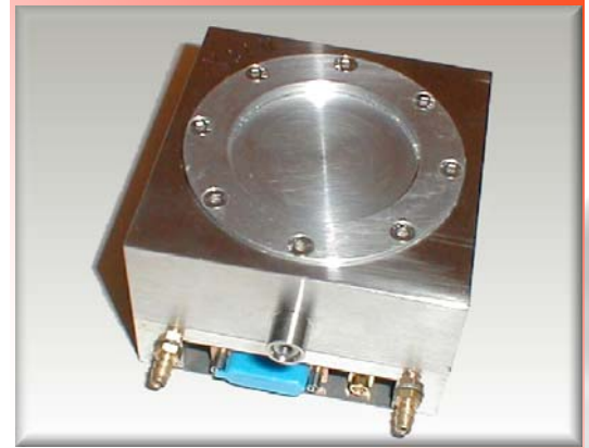
Figure 1 The CCD camera head housing a CCD bonded to a scintillating fibre optic plate (SFO), supplied by Xcam Ltd.
