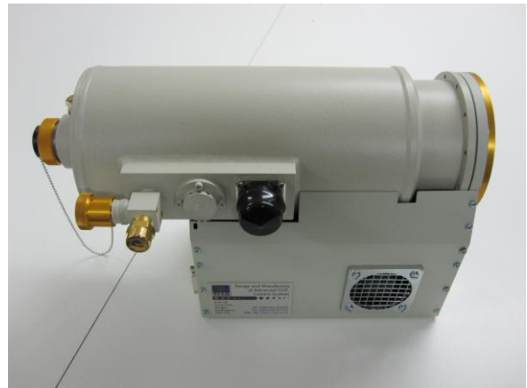
Figure 5: Images of the CCD Camera System showing each side (top left and top right) and the liquid nitrogen entry port (bottom left); front face image shown in figure 1.
