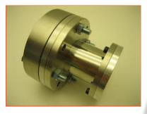
The device used was an uncoated, back illuminated e2v technologies CCD97 with 512 x 512 x 16 micron pixels. The devices had no AR coating as is standard for this device, and XCAM produced a mechanical shield to enable frame transfer operation in the absence of the aluminium shield.
