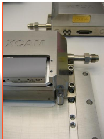
Figure 2 XCAM Single Unit on Base Plate in Foreground with Sensor Exposed to view, and (background) Alternative Orientation
